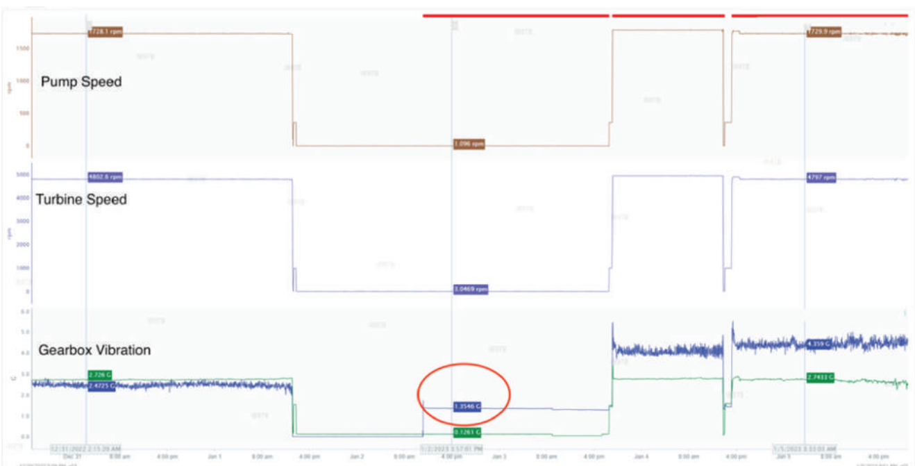
Figure 2: Faulty Accelerometer Readings of a Gearbox
